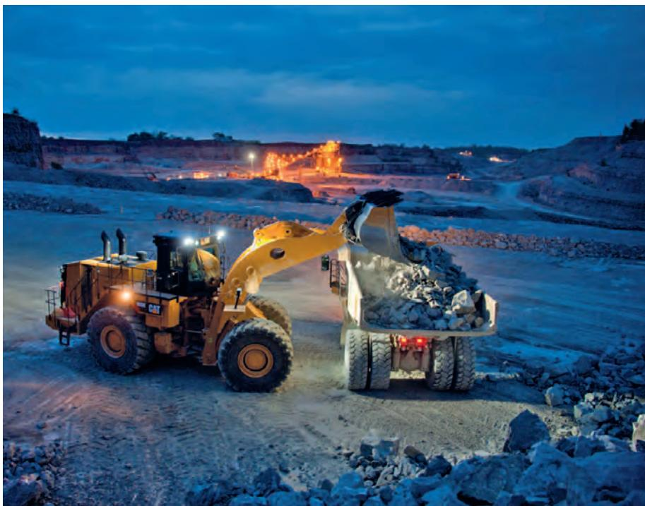
range. The operator has full control over the load for increased safety and productivity. Double seals on all linkage pins retain lubricating grease and prevent dust for outstanding durability and long machine life, and the TP linkage geometry provides excellent bucket roll-back angles for increased stability and less spillage.
