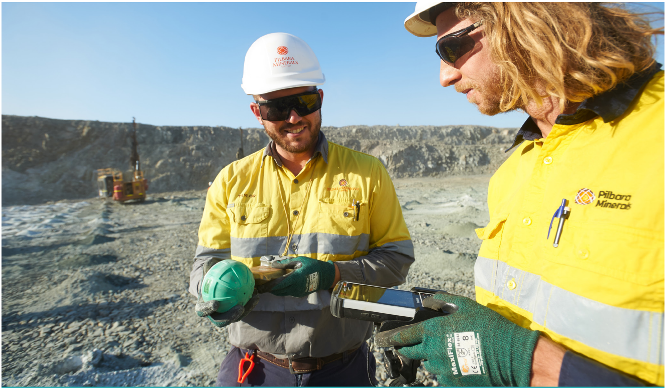
Blast movement monitoring and analysis collects data from blast movement sensors, which move with the blasted material. Software is used to transform the data into actionable insights – from the post-blast location of ore to creating more precise dig lines based on the measured movement. Photo: Hexagon.
