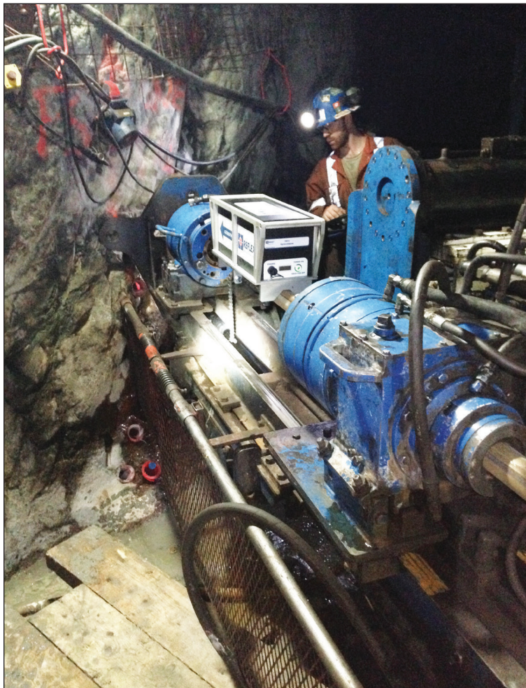
Reflex TN14 Gyrocompass installed on a rig
