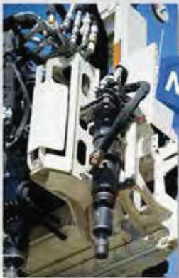
High-Speed Sonic Coring Head
