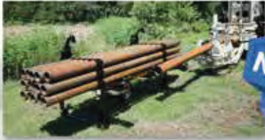
Indexing Rack for 10-ft. Sonic Tooling
