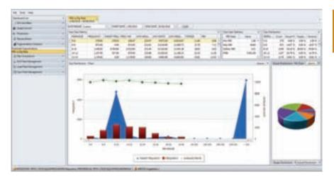
HxM Athena features dashboards showing the predicted fragmentation distribution curve versus the measured actual fragmentation curve, and compare them to the digrate of the excavators; a valuable tool for planning engineers
