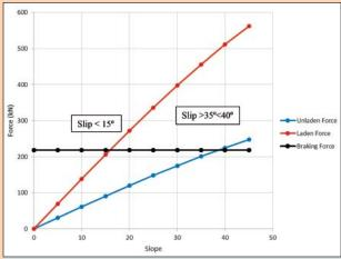
Determining the force of loaded and unloaded trucks on a downhill slope can pinpoint the gradient at which wheel-locking interventions could cause slippage. (Image: Kaelo, Olehile; et al.)
