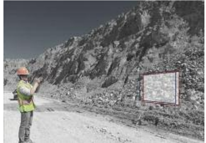
A major advantage of using PortaMetrics is its ability to provide point and shoot fragmentation analysis of a desired scene in seconds
