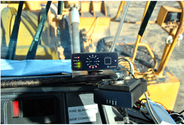
Figure 2. Taking up minimal room on the dashboard, the size of Hexagon's collision avoidance system belies its importance to the protection of both the operator and vehicle.
