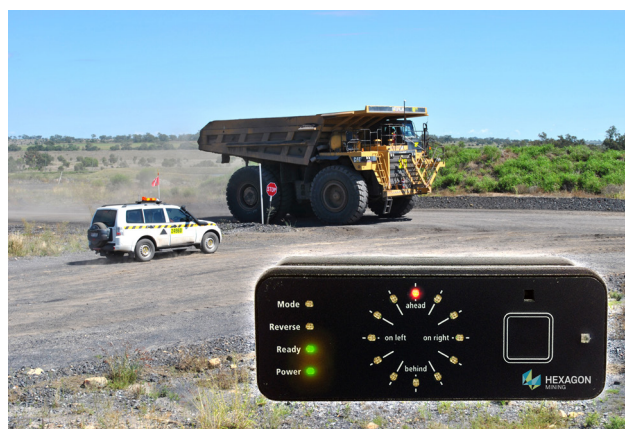
Figure 6. CAS monitors 360° around the vehicle and vehicle locations are indicated on an LED display for intuitive manoeuvres on its visual line of sight.
