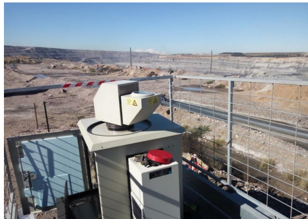
Figure 5. A mini micro-pulse LiDAR instrument in an all-weather enclosure deployed at HVO in New South Wales.
