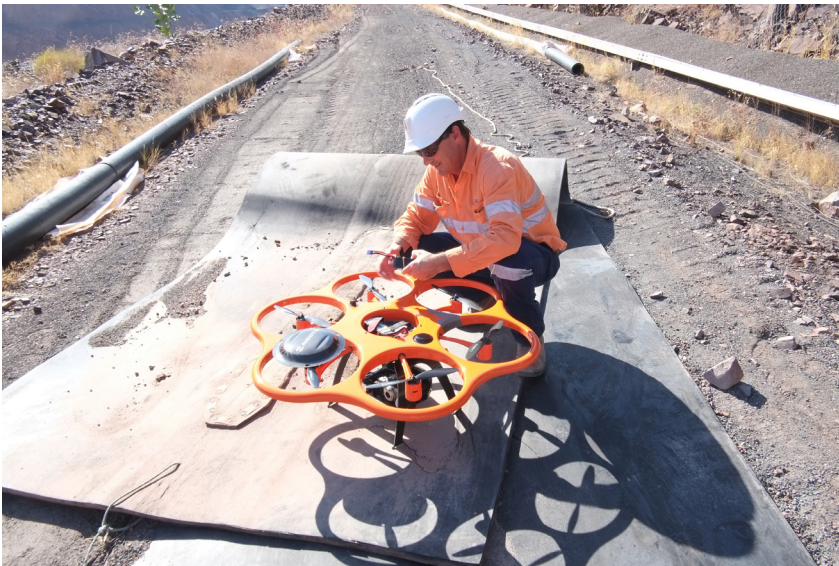
Autonomously flying hexacopters, such as the Aibot X6, are pushing the boundaries of photogrammetry. 2
