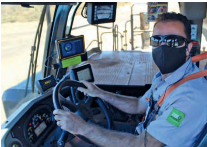
Operator at Mineração Usiminas (MUSA) iron ore mine in Brazil using Optalert glasses-based fatigue monitoring system
