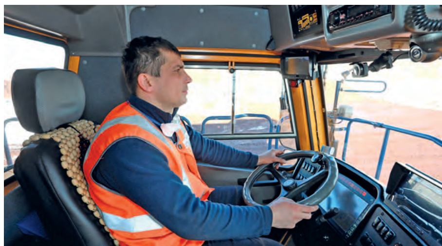
Operator being monitored by OKO Mining camera based system in 240 t BELAZ truck at Metalloinvest's Mikhailovsky GOK iron ore mine in Russia
